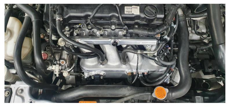
23. Your Plazmaman Fuel rail is designed to suit full length injectors out of the box, if you choose to run the OEM injectors you will need to either cut the fuel stands down 12mm or use ¾ – full length injector extensions. We designed it this way so to give more options in terms of injector choice.
