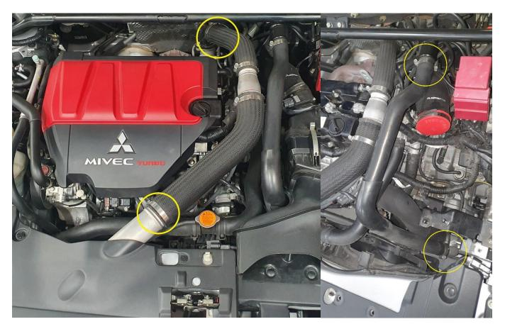
5. At this stage it is recommended you block all openings into your engine, Intake pipe, turbo outlet, intercooler pipe above your radiator, both ends of the BOV recirc system, and lower cold side intercooler pipe. <u>Failure to</u> follow this step may result in engine damage due to debris, tools or anything entering the engine.
