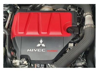
3. Now remove the airbox and MAF, you will find 2 plastic push rivets holding the air dam in place, 2 retainer clips on the top of the airbox, 1 single hose clamp attaching the MAF to the intake hose, 1 Electrical connector to the MAF with 2 harness retaining push clips and 1 single 10mm bolt to the right side of the airbox. See the pictures below.
