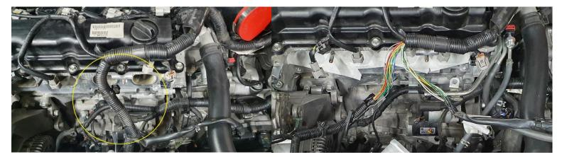
16. Rotate the longer water hard-line on your throttle body to point in the direction shown below in the second picture or remove completely. We choose to delete this waterline during the process of installation, by looping the water line at the motor.
