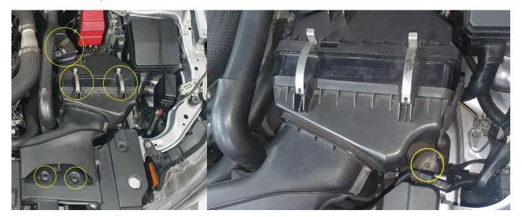
4. Remove the BOV (blow of valve) recirculating hose, hot side intercooler hose that runs from your turbo and intercooler hose which runs into your throttle body – each will require removal of a hose clamp at either end.
