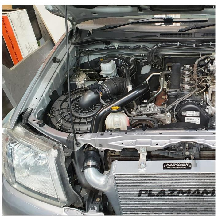
21) On the passenger side, remove and replace this m6 shroud bolt with the new dome head hardware.
