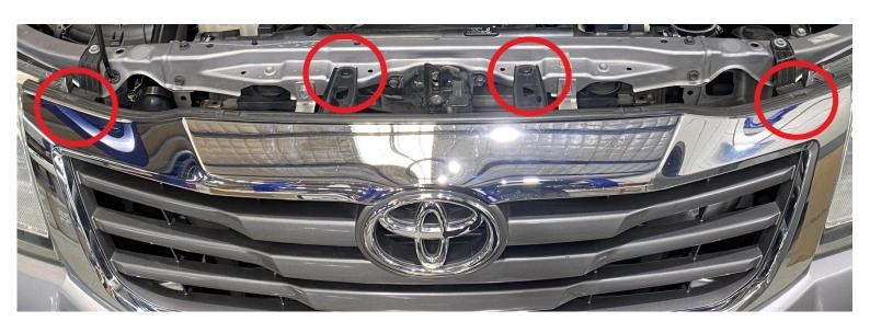
6) Remove plastic inserts beside both head lights and unclip the wiring from centre support brace and horns.
