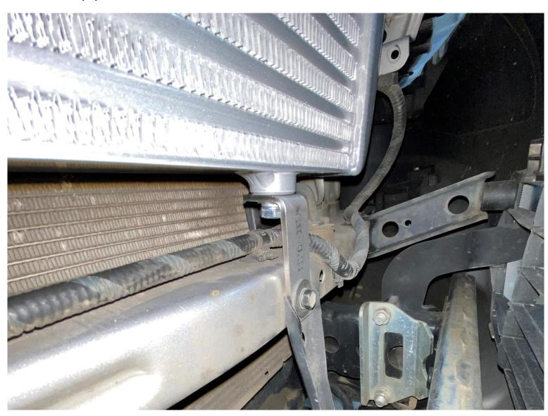
19) Loosely bolt the top intercooler brackets one side at a time by adding them in front of the horn brackets. (Be sure to support the horn while you carry out this process, so it doesn't fall)
