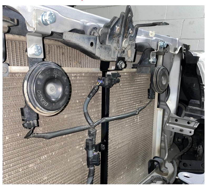
15) Using 4X supplied M8x16 hardware loosely bolt top and bottom intercooler brackets to Plazmaman intercooler in the orientation shown in pictures.
