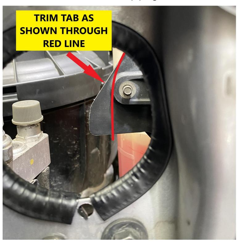
12) Bolt in the new supplied rad support brace with bonnet latch. Ensure factory bolts are used in their original positions.
