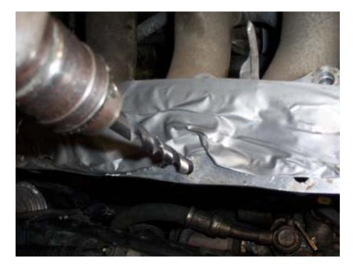
3. Drill out x2 threaded holes with a 8.5 – 9mm drill bit. THE HOLES MARKED WITH AN ARROW BELOW
