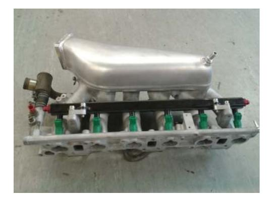
6. **FITTING OF INTAKE PLENUM** - Must use gasket, either reuse OEM if in good condition or a new replacement must be purchased.
