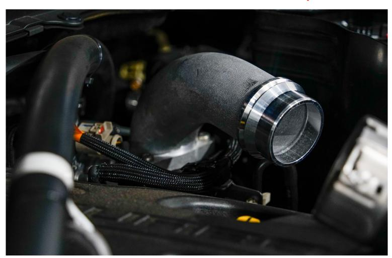
10.Install the supplied circlip adapter fittings to the turbo outlet and throttle body elbow. Install the supplied wire circlips to the adaptor fittings.
