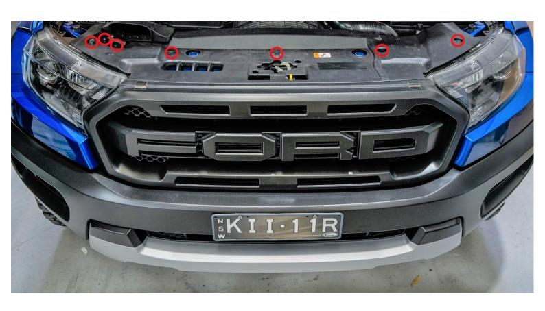
Now lift the rear of the diversion panel and reach underneath into the grill section. Carefully unclip the 6 hidden tabs that attach the front of the diverter panel to the front grill.
