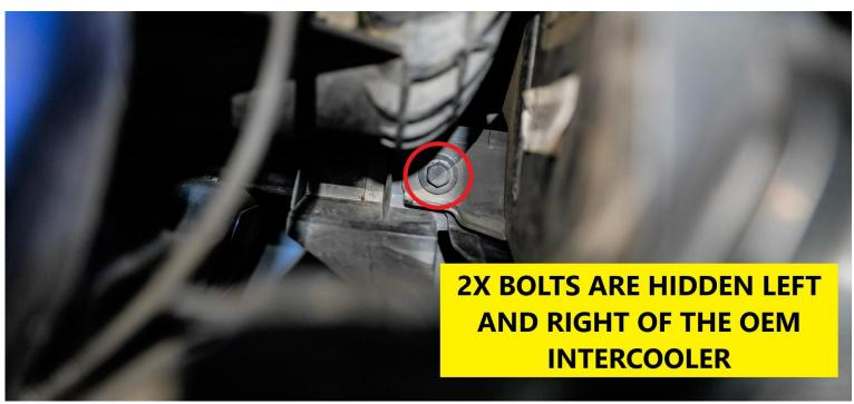
3. Removing of the secondary air divertor located on top of the OEM cooler.
