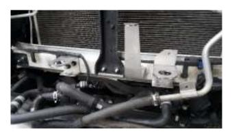
17. Disconnect both water pump's electrical plugs.
