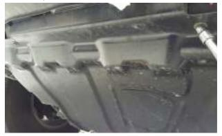
2. Release the FOUR remaining clips retaining the side intercooler ducts and remove.
