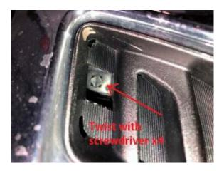
6. Release the SIX tabs hidden behind the front grill while pulling the grill forward to release it from the radiator support.
