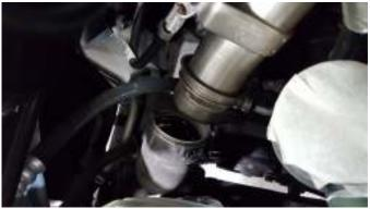
10. For the cold side, simply undo the hose clamp on the hose. The intercooler should now be easily removed from under the vehicle with the factory hoses still attached to the intercooler.
