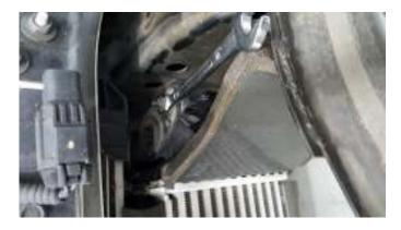
7. Remove the FOUR 13mm bolts holding the intercooler bracket to the chassis rail and remove.
