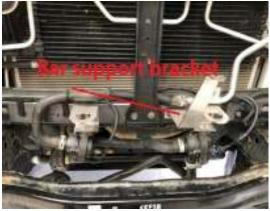
15. Install the Plazmaman hard line support bracket in between the chassis crossmember and passenger side intercooler bracket.
