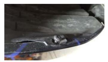
4. Pull the plastic from inside the wheel well away from the front bumper to expose the 10mm bolt holding the bumper to the guard and remove.
