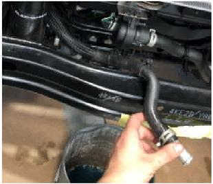
23. Once cut, the hose can be reconnected to the U hose using the original Nissan hose joiner and clamps. The hoses should sit naturally with no kinks.
