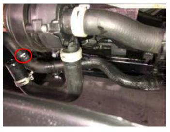
22. Cut the LONG driver's side water pump hose at the white line in the above and below pictures. The cut should be approximately 3 BENDS BACK from the original hose end. A hose cutter should be used to ensure a clean, straight cut.
