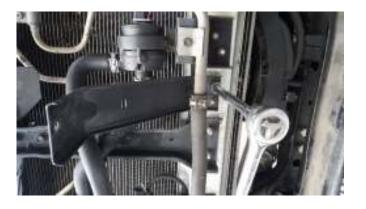
12. Remove the FOUR steel clips holding the rubber mounts to the brackets. Retain for later.
