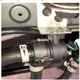
21. Disconnect the driver's side water pump hose from the hose join in the factory plumbing as pictured below.
