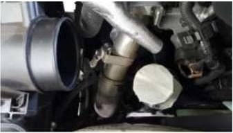
Using a flat blade screwdriver, gently pry the circlip into the locked open position, repeat for the opposite side of the coupling. Take care to not use excessive force, the pipe should pull away easily.
