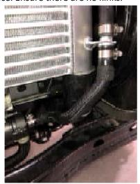
33. Connect the supplied 19mm hose to the factory hard line near the headlight, and the opposite side of the hose barb located on the intercooler tank. The connection should look as pictured below. Fasten the hose with a Nissan clamp at the headlight end, and a supplied hose clamp on the intercooler end.
