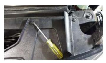
2. Remove FOURTEEN bolts from the bottom of the bumper and stone.
