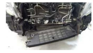
1. Remove the TWO 10mm bolts holding the stone tray and remove.
