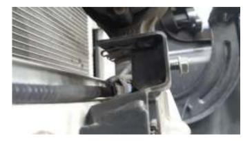
13. Remove the FOUR 13mm nuts holding the pump brackets and remove the brackets, retain the nuts.
