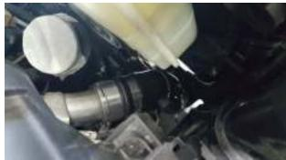
32. Connect the previously removed passenger side water pump hose and reconnect it to the passenger side water pump in the **REVERSE**ORIENTATION. The hose should line up with the barb fitting on the passenger side intercooler tank as shown below. Use the supplied hose clamps to tighten the hose in place. Ensure there are no kinks.
