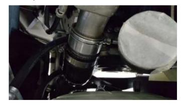
31. Remove the tape covering the turbo inlet and install the factory air intake hose or Plazmaman hose if purchased separately and tighten clamps.
