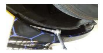
5. Using a flat blade screwdriver, turn to unlock the FOUR plastic fasteners hidden inside the front of the grill.
