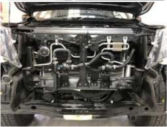
9. Release the FOUR clips from the sides of the intercooler duct and remove.
