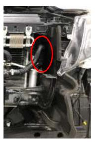
20. Secure the water pumps upside down to the new Plazmaman water pump mounts using the previously removed clips.
