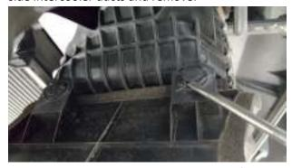
3. Remove the TWO 10mm bolts holding the fan shroud to the intercooler.
