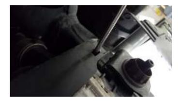
6. Remove the TWO 13mm nuts from the top intercooler brackets.
