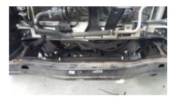
11. Remove TWO 10mm nuts holding the centre bar support and remove. \*Note\* Series 4 models do not have the coolant hard line pictured.
