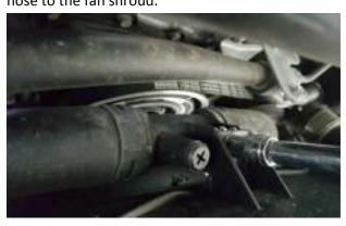
5. Pry the fan shroud retaining clips away from the intercooler to release.
