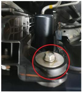
• You will need to bend the small bracket on the bonnet latch for the wiring harness to clear the intercooler, after this check that the bonnet latch clears the intercooler.
