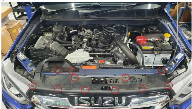
3. Now remove the grill by releasing the retaining clips from the top, you will also find a single Philips head screw in the front of the grill. See below.
