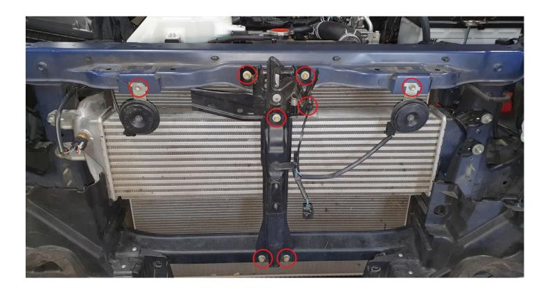
10. Take your intake pipe, hot and cold side intercooler silicon's off the car, you will have one hose clamp on each side of the silicon. After this remove the air temp sensor and 4 bolts holding the OEM intercooler.
