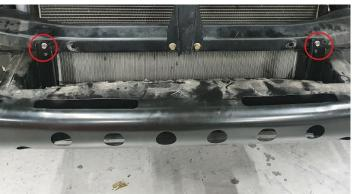
9. Remove the centre radiator support structure, bonnet latch and horn.
