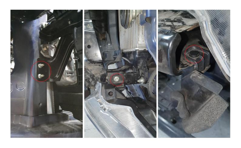
8. Remove the 2 plastic retaining clips on the lower air diversion plate and remove the 2x 10mm bolts holding the 2 bumper support straps on either side of the air dam, this will need to be done before you can remove it from the vehicle. See below of the bolts hidden location illustrated with the air dam removed.
