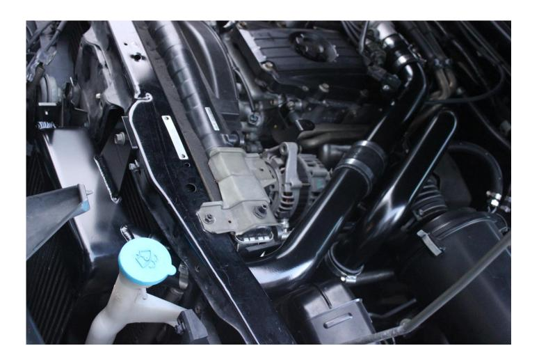
10. Piping can now be fitted. Both hot and cold side piping should be fitted in a way where it does not have a chance to rub against any metals as this could lead to issues later on. Once the lower piping is fitted and routed past the wheel section, you will need to test LOCK-TO-LOCK steering of the vehicle, to check wheel and tire clearance. This is critical for raised vehicles, or for vehicles with over size tires. See below some piping fitting pictures as a guide.
