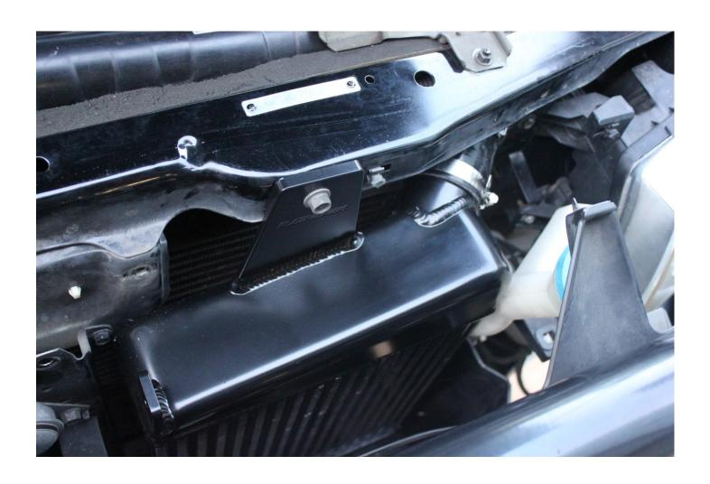
8. Once intercooler is bolted into place you now can go ahead and fit the power steering cooler back onto the side of the intercooler. There is a mounting provision for this. You will need to loosen the bolts for the steering rubber mounts and bolt into place similar or as per the x2 pictures below.
