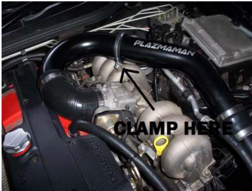
10. Fitting of the HOT SIDE pipes
