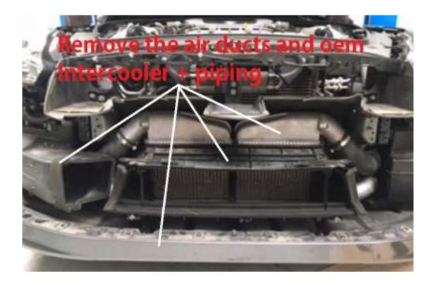
4. AIR DUCT RE INSTALLATION PROCESS – The Plazmaman GTR35 Intercooler kit takes full advantage of re-using the OEM factory air ducts. Since the RIVETS were drilled out to remove the air ducts, you must now reinstall some M6 NUT-SERTS that we supply - X4 in total. You will require a NUT-SERT tool for this. AT THIS STAGE DO NOT INSTALL THE AIR DUCT.
