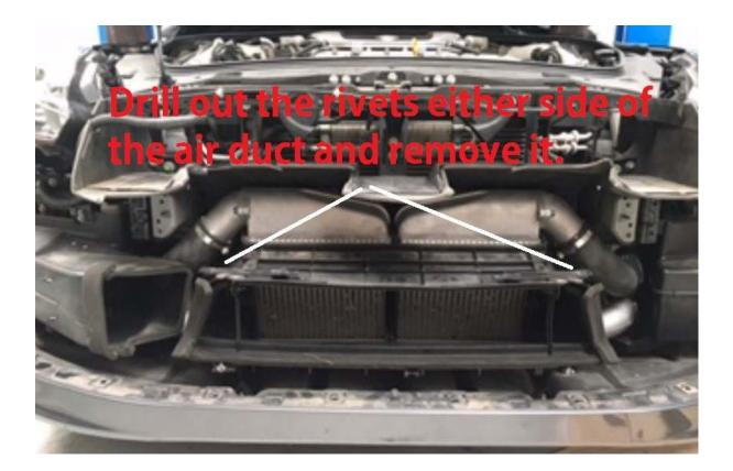
3. Then remove the factory Air intakes, Intercooler piping and factory Intercooler. You will be reusing the OEM Intercooler mounting locations and Bolts. DO NOT MISPLACE THESE.
