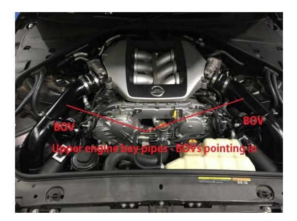
8. Once the upper piping has been installed via the intended route, now you must refit the OEM BOVs, including the plumbback hoses, or if you have aftermarket items, they must be fitted as per normal BOV operation design. Add the BOV vacuum hoses to the BOVs. Next install both the sensors in either pipe as per below picture. Plug in the loom plugs to each sensor once mounted.
