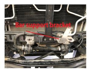
30. Install the Plazmaman hard line support bracket in between the chassis crossmember and passenger side intercooler bracket
