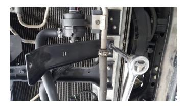
21. Undo the 10mm bolt holding the water hose hard line the passenger side pump bracket. Retain the bolt.
