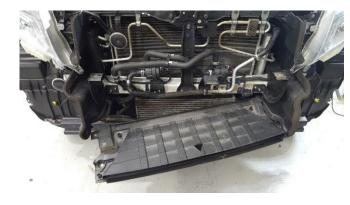
10. Remove the TWO 10mm bolts holding the stone tray and remove.
