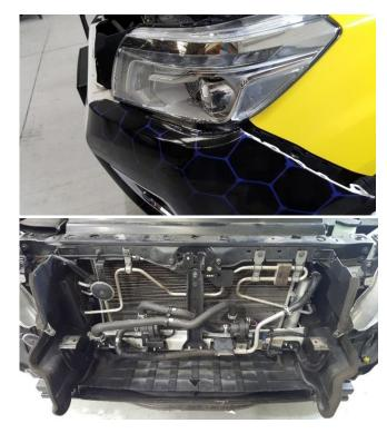
9. Release the FOUR clips from the sides of the intercooler duct and remove.
