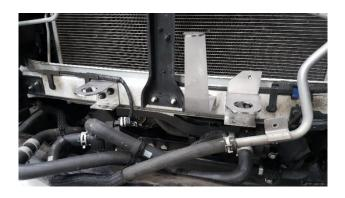
32. Fasten the hard line to the hard-line support bracket.
