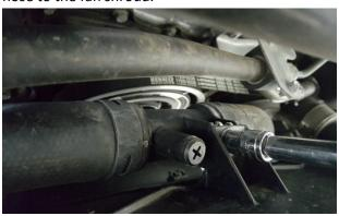
14. Pry the fan shroud retaining clips away from the intercooler to release.
