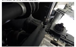
13. Remove the 10mm bolt holding the radiator hose to the fan shroud.
