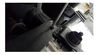
15. Remove the TWO 13mm nuts from the top intercooler brackets.
