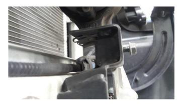
24. Remove the FOUR 13mm nuts holding the pump brackets and remove the brackets, retain the nuts.
