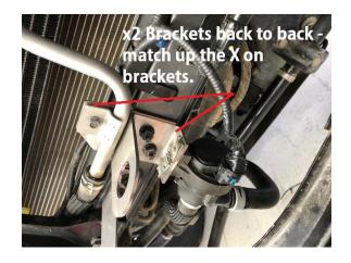
31. Install the Plazmaman intercooler support bracket, these are side specific.
