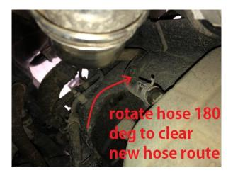
42. Fit the Plazmaman hot and cold side hose with the supplied hose clamps and tighten, make sure that none of the hoses rub any other parts.
