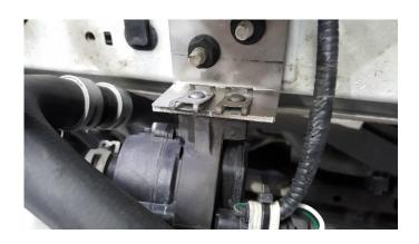
34. Install the supplied 2" P-Clamp on the rearward end of the Plazmaman hose support bracket, just under the a/c condenser
