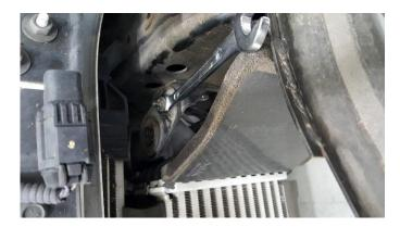
16. Remove the FOUR 13mm bolts holding the intercooler bracket to the chassis rail and remove.
