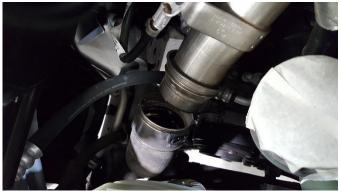
19. For the cold side, simply undo the hose clamp on the hose. The intercooler should now be easily removed from under the vehicle with the factory hoses still attached to the intercooler.
