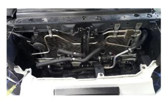
9. Carefully pull the bumper away from the headlight area to release it from the vehicle, this should be done simultaneously on both sides with two people. Disconnect the front fog lights when the bumper is pulled away.
