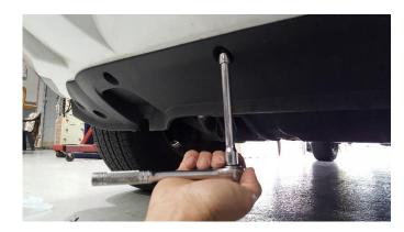
Remove screw from inside of the wheel well. Repeat for other side.
