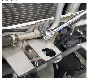
33. Disconnect both water pump electrical plugs and fit both water pumps to their corresponding Plazmaman brackets and install the factory retaining clips.
