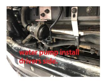
BEFORE CONTINUING TAKE THIS TIME TO ENSURE THAT THERE ARE NO KINKS IN THE HOSE SYSTEM, SKIPPING THIS STEP MAY LEAD TO MECHANICAL DAMAGE.
