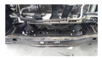
20. Remove TWO 10mm nuts holding the centre bar support and remove.
