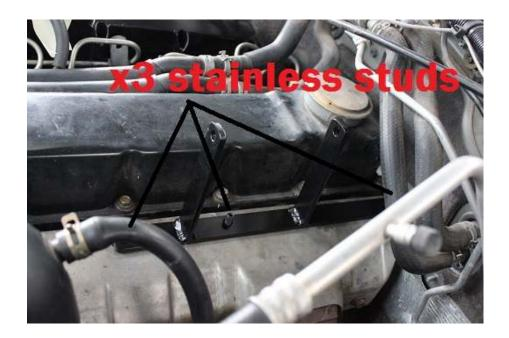
9. Now carefully pick up the W2A unit and test fit over the x4 upright brackets. The uprights sometimes might have to be tapped in or outwards to suit the w2a width. This can be done carefully with a plastic hammer. Once the w2a unit is in place, bolt it into place and make sure you tighten the x3 nuts on the top part of the exhaust manifold bracket.
