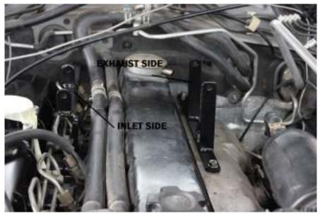
Plazmaman P: 02 9725 1728/ F: 02 9725 1722 www.plazmaman.com 8. The bracket on the exhaust side is a lot easier to fit. Using the supplied stainless studs, screw them into place tightly where the original bolts through the heat shield used to go. Fit the bracket and add the nuts/flat washers, but do not tighten yet.
