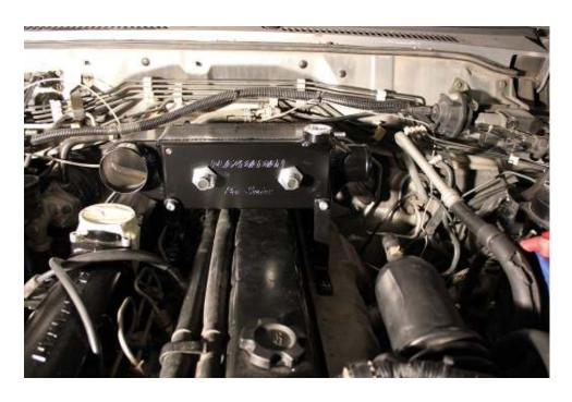
10. Next step is to add the turbo side and inlet entry piping. The inlet side is standard across all models but the turbo side will sometimes vary due to different models and aftermarket turbo setups that are around. We can cater for all setups but sometimes need feedback to get them correct.
