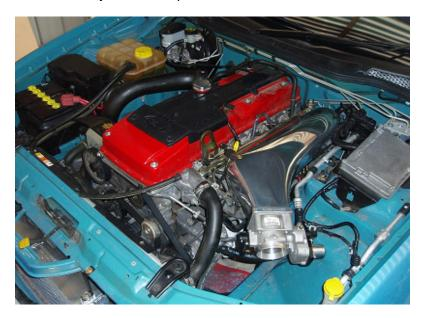
12. Use a flexible silicone joint off the throttle body. (There must be ample movement of this first hose)
