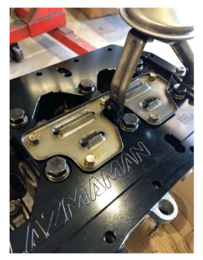
9. This baffle must be removed from the sump before installation.
