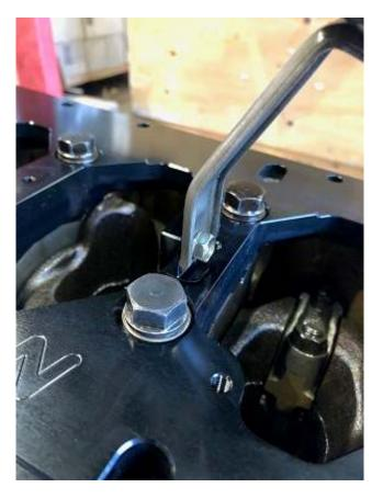
8. Install the factory windage tray using the factory bolts.
