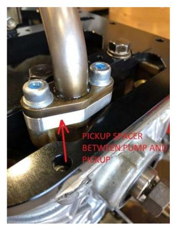
7. Attach the oil pickup to the girdle using the factory bolt.
