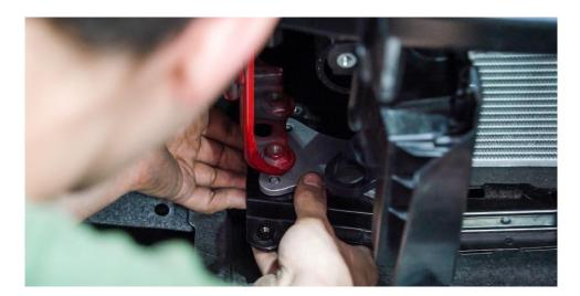
9. **Optional:** If desired, trimming of the oem plastic intercooler shroud may present the intercooler better for a cleaner look. On the passenger side, be sure to leave the mounting hole for the air temperature sensor intact (circled in red).
