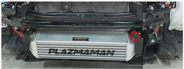
10. Your new Plazmaman intercooler is now installed. Follow these instructions in reverse for reassembly. There should be four 12mm bolts, three plastic clips, the lower intercooler shroud and the oem intercooler left over once reassembly is complete.
