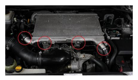
3. Remove the 2x 10mm bolts holding the engine cover retainer, you will need to reuse this retainer if you want to retain the engine cover.
