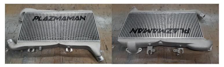
2. Fit the OEM rubber bushing and sensors onto the new Plazmaman intercooler.
