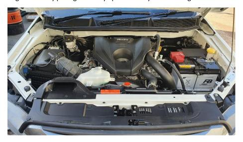
2. Now you will have access to the plastic OEM throttle body pipe prone to cracking. To remove this, you will find one electrical connection to the left side of it, three 10mm bolts and 2 hose clamps.
