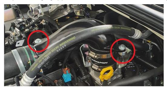
5. Reinstall the cold side silicon joiner to the front outlet of the Plazmaman throttle body pipe. Tighten all three hose clamps, plug the sensor back in and you are done with the installation.
